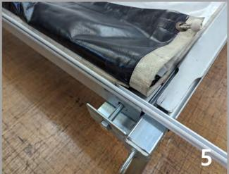
**Step 8:** Flip the front flap of the roof up onto itself to reveal the keder bead which is attached to the inside. You just need to make sure the front beam is bolted loosely to make sliding the joining strip in the front top groove and the bead on the roof easy..
