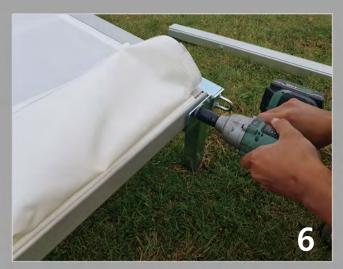
**Step 9:** When the Joining Strip is entered into the Tension Beam 'H' and is slid all the way across you can tension using Bolts Ic, these 130mm bolts are inserted from the front and located into the captive nut on the reverse of the Tension Beam 'H'. Once installed with your fingers, you will be safe to pull up with a socket driver as shown in Photo 6. Warning - Do Not Over-tighten!
