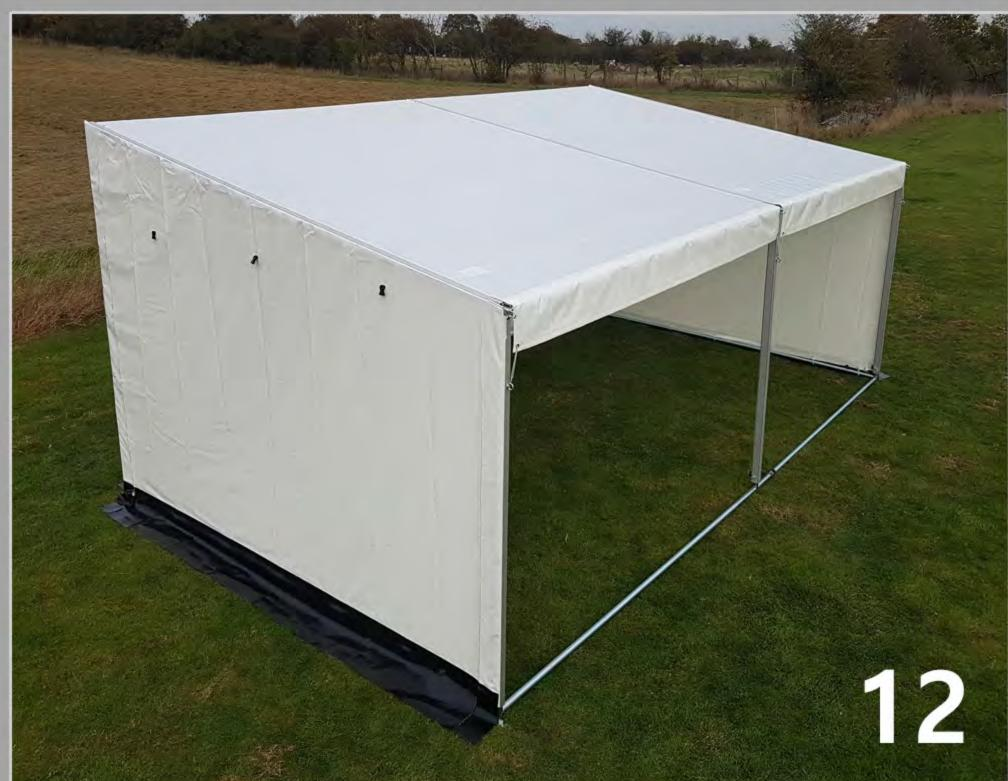
**Step 11:** Slide the side walls into the top outside groove of the Main Beam 'F', when you have the wall slid all the way up to the top, open the zips and slide the edge with the keder bead into the leg and do up the zip.
